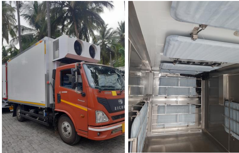
Figure 5: (L) 14 feet frozen reeper truck (R) Inside view of reeper truck – PCM plates lined on inner walls of truck
