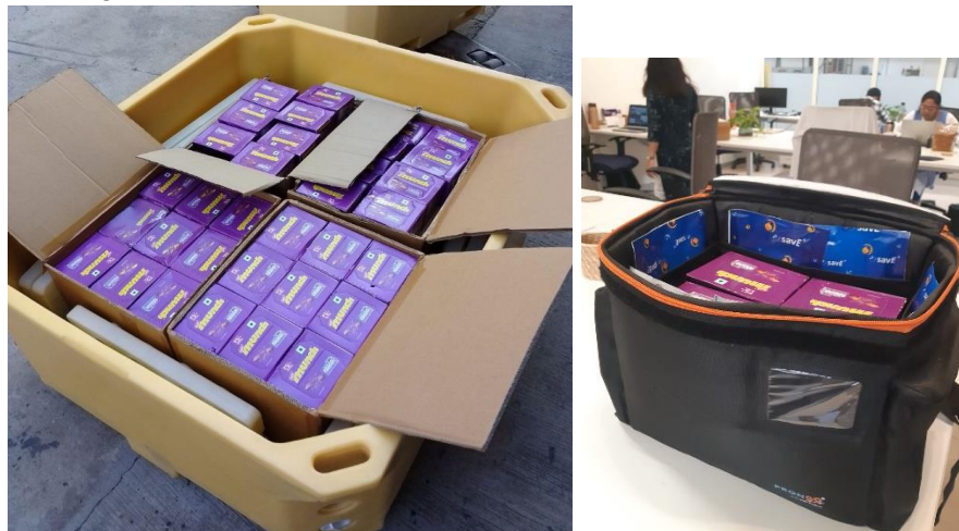
Figure 1: Storage of chocolates in (L) Rotomoulded box with PCM tabs (R) Soft bags lined with PCM pouches
