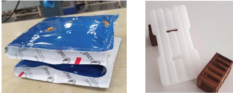
Figure 3: (L) PCM pack (R) PCM plastic tab
