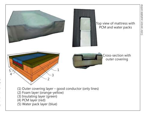
**Fig. 1.** Construction of the PCM bed. The bed consists of an outer covering made of nylon (1), a hollowed-out foam layer (2) lined with an insulating material like extruded polystyrene (3), PCM blocks kept in the hollowed-out area (4) and a water mattress above the PCM blocks and below the outer covering (5).
