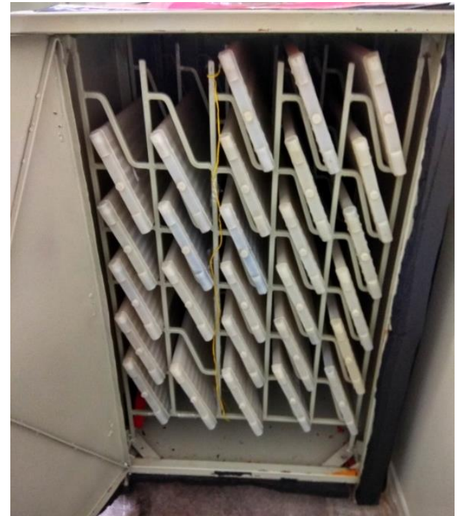
Figure 12(a) PCM air HX closed view (b) Stacking of the HDPE extruded panels inside HX open view
