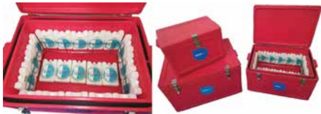
Figure 3: Thermally insulated boxes lined with PCM thermal battery of the PCM material completely. A PCM material's core utility is derived from its ability to store latent heat at the designed temperature. Latent heat is the energy absorbed or released during phase transition, for instance, if the PCM thermal battery contains a (-)26C Cell material then it needs enough cooling energy at a temperature lower than (-)26C Cell to ensure freezing. A PCM thermal battery provider hence would provide the right charging unit as shown in figure 2.
