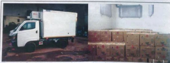
Figure 3: Partially electric refrigerated truck with TES (Image courtesy: Pluss Advanced Technologies)
