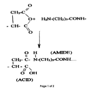
Under conditions of average performance of an injection moulding machine, with L/D ratio of 20, the plasticizing screw and passage of the melt through the injection nozzle gives adequate mixing and residence time for a chemical reaction to take place between amine end-groups of Nylon and anhydride groups on OPTIM<sup>®</sup>. It is these chemically bound polyolefin chains that are responsible for the substantial improvement in impact strength of Nylon by way of alloy formation.
